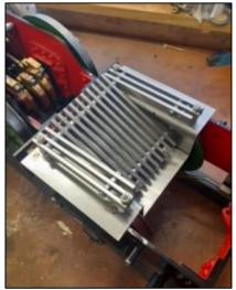
added washers as packing to get the necessary spacing all in stainless steel.
