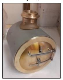
cut so I could hold it a 3-jaw chuck whilst I turned it to length. Used castings for the smokebox door and ring. The hinges for the smokebox door pushed my model making skills to the limit, not perfect but the door opens and closes as it should, what more can I ask.
