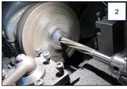
be remade. This is one of the first replacement things that I did. **Picture 2** shows a replacement eccentric being machined.
