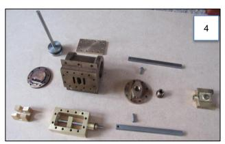
the ports and one of them drifted off a bit, but ultimately, they seem to be satisfactory. The valves still need more polishing to slide on the valve plates, but otherwise the cylinder components are largely complete as can be seen in **picture 4**.
